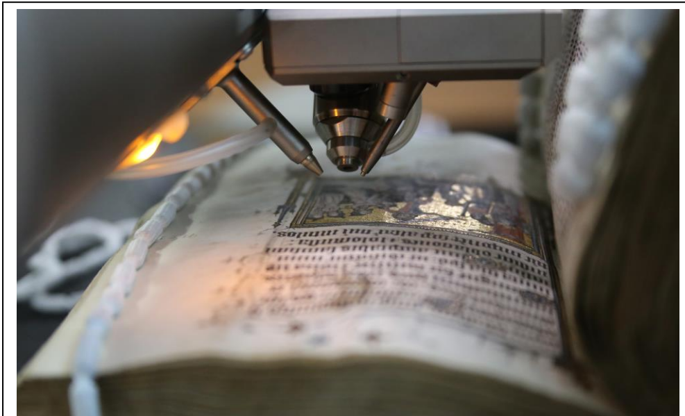
XRF Analysis of an Illuminated Manuscript at the Fitzwilliam Museum, University of Cambridge.
